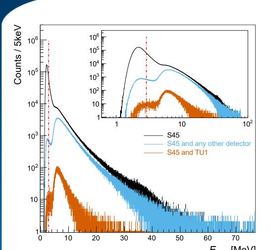
Signals in panels need to have a threshold energy and maximum time difference to a signal in TU1 in order to act as veto signal.
