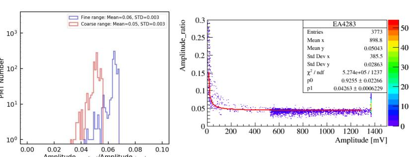
The amplitude between signal and overshoot of the two ranges are about 6% and 5%.
