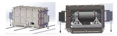
A 20 cm thick lead shield is placed around the detector to stop the  $\gamma$  rays
