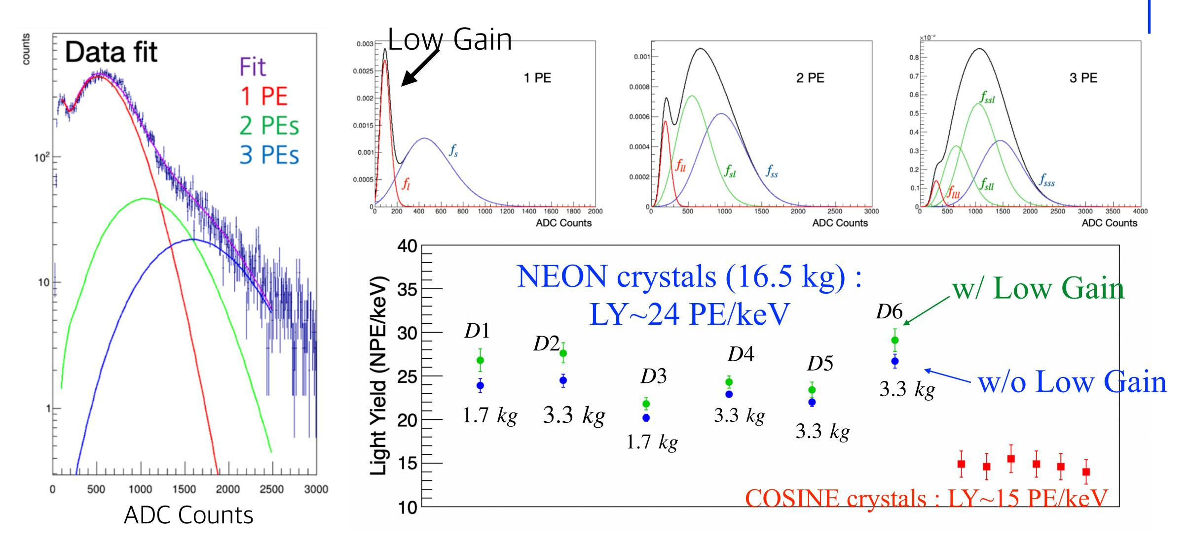
NEON crystals show high light yields (size matching & simpler coupling)
