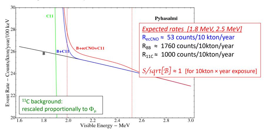
Signal comparable to stat. fluctuations for exposures 10 kton × year or larger.
