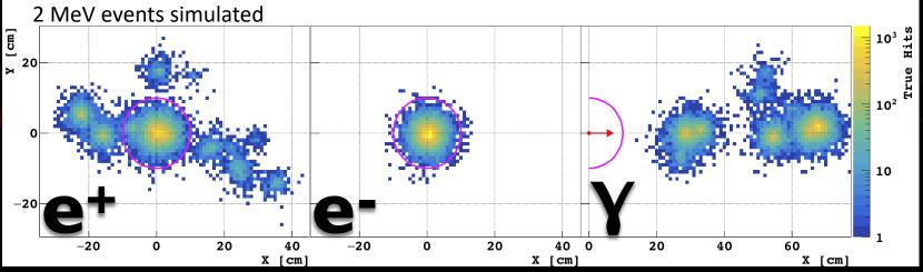
short light scattering length stochastically confines scintillation photons energy deposition pattern can be imaged by collecting light with grid of wavelength-shifting fibres
