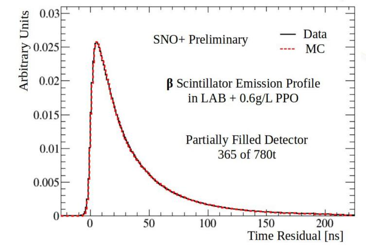
The plot presented above shows the time residuals of <sup>214</sup>Bi decays, tagged by their coincidence with daughter <sup>214</sup>Po decays in partially filled detector, demonstrating detector calibration and agreement in position reconstruction between data and Monte Carlo.
