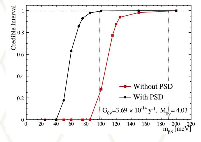
Finally, instead of mere hard cuts, the classifier values can also be used as additional dimensions in likelihood fits. The  $0\nu\beta\beta$  3 year sensitivity with 0.5% Te is plotted on the left, showing significant discovery potential improvement when PSD is included in the fit.
