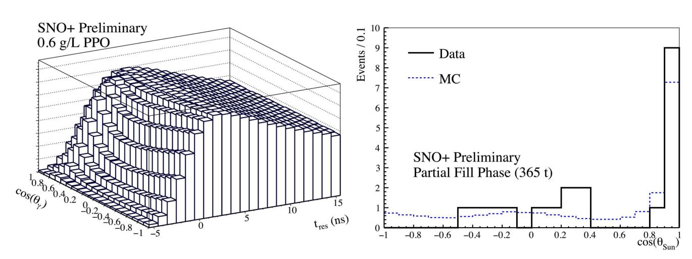
$\theta_{y}$  = angle between event direction and hit PMT with respect to event position  $\theta_{y}$  = angle between reconstructed event direction and direction from the Sun
