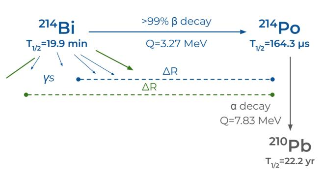
The technique was validated by applying the classifier to tagged  $^{214}$ Bi decays in partially filled detector (365t of LS).  $^{214}$ Bi with more spread-out energy depositions reconstruct on average further away from the daughter decay. The plot above shows that these with higher  $\Delta R$  have lower discriminant values as expected and presents the first data-driven demonstration of this technique.
