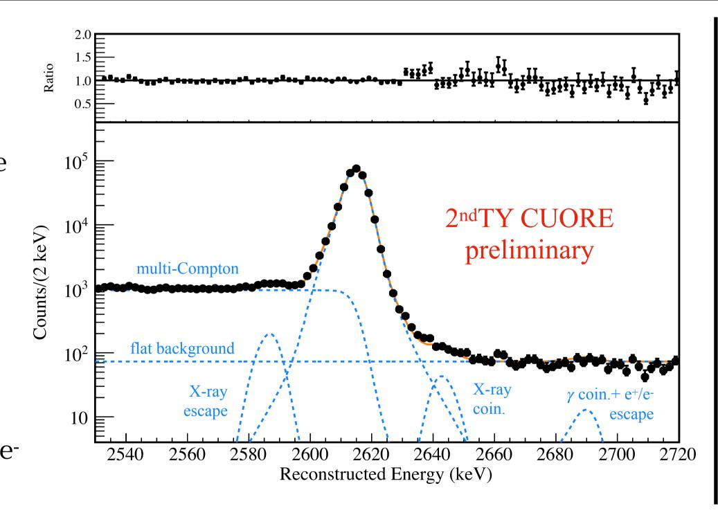
• peaks in the *background spectrum* are fit with the 2615 keV-calibration-based line shape to determine the detector response parameters in the region of interest (ROI)
