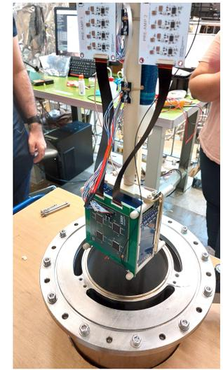
Insertion into cryostat
