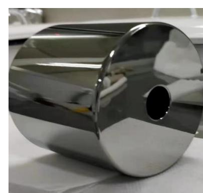
ICPC: Inverted Coaxial Point Contact
