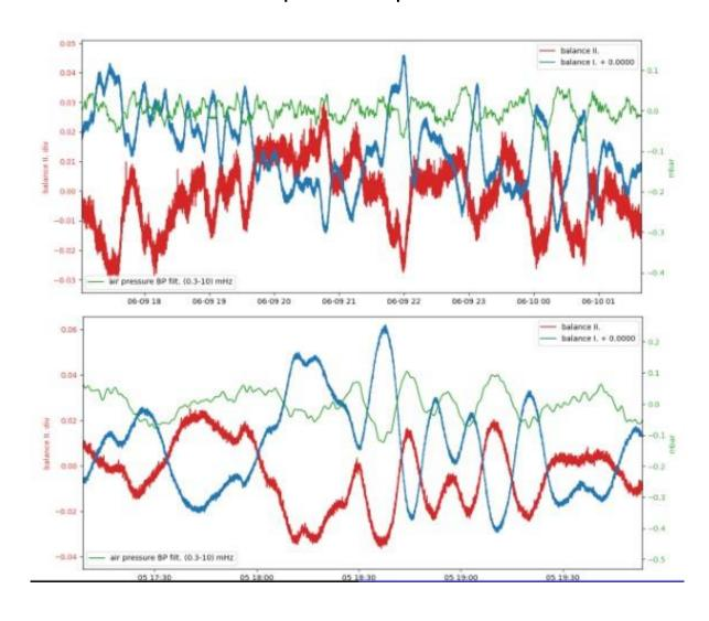
The changes of atmospheric pressure cause the tilt of the ground below the balance
