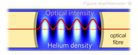
superfluid <sup>4</sup>He filled optical cavity
