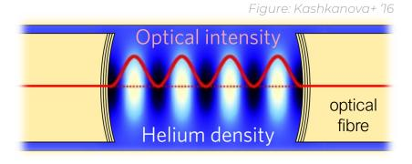
superfluid <sup>4</sup>He filled optical cavity
