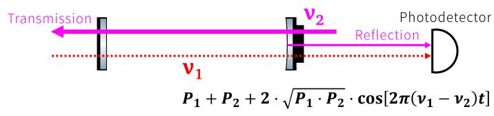
Detection of a 2-photon-per-day flux
