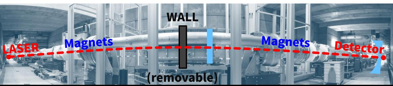
Production Cavity is absent -> 40 times more light on the COB, facilitates stray light hunting
