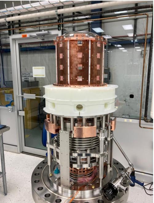
Quartz blocks LAr scintillation. The addition of the Xe waveshifts aids in the transmission and collection.
