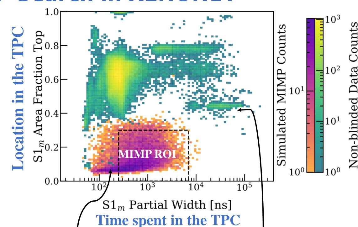
Backgrounds: BiPo decay chain, detector artifacts, muons (99.5% veto) MIMP signal: clustered S1s ( $S1_m$ ) with a time scale around  $1\mu s$ .
