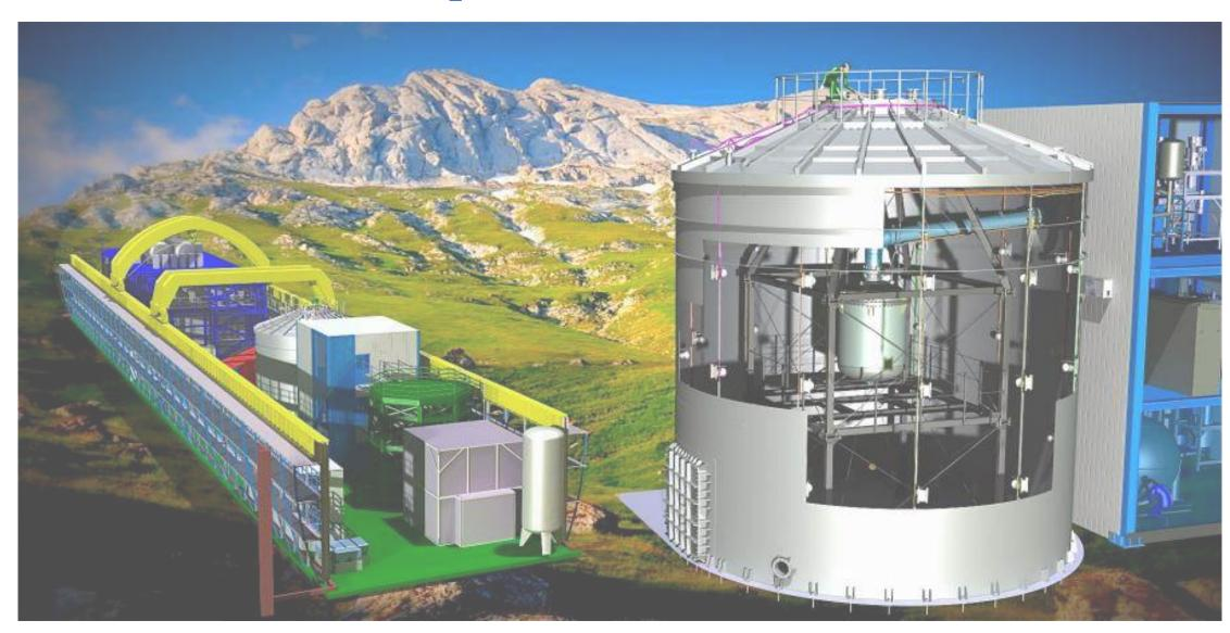
XENON1T use a dual phase time projection chamber (TPC) filled with 3.2 tonne of ultra-pure liquid xenon (LXe) located at INFN Laboratori Nazionali del Gran Sasso under 3600 m water-equivalent overburden.
