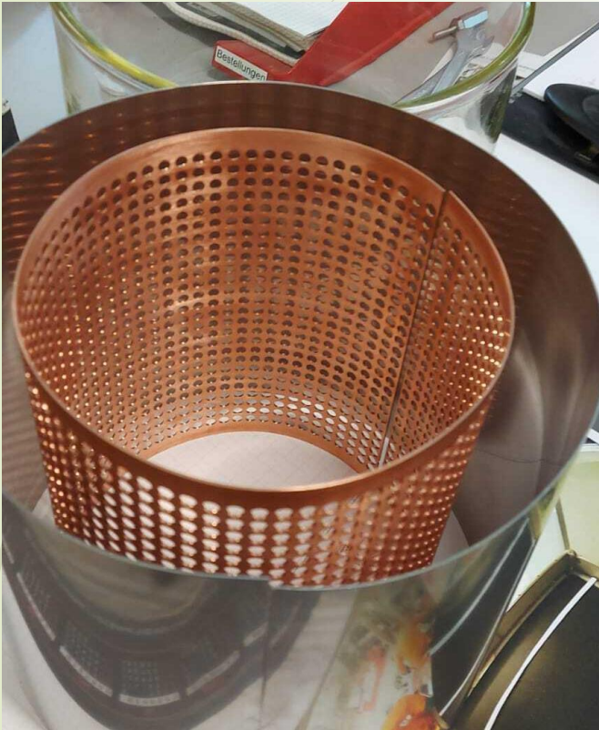
New electrode design for coating of cylindrical vessel
