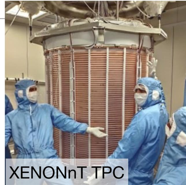
Particles interacting in a noble liquid Time Projection Chamber (TPC) create scintillation photons (S1) and ionisation electrons (S2).
