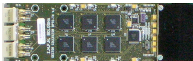
Figure 3: The OPTO-TX mezzanine.
