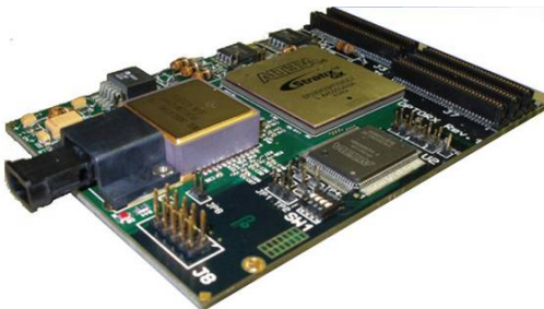
Figure 4: The OptoRX12 mezzanine module
