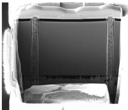
Figure 9a-c: Schematic (top) and FIB-graph (bottom) of a 3D-integrated test stack with daisy chains
