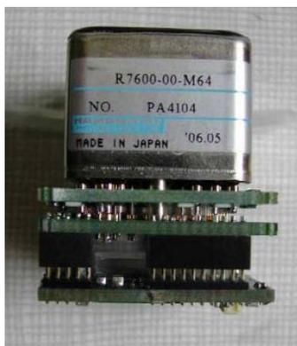
**Figure 4: photomultiplier front-end module (PMF).**
