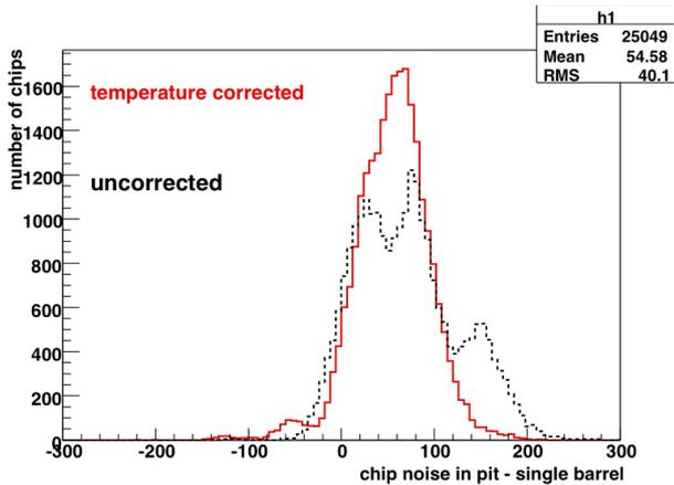
Figure 4: Comparison between the average input noise per chip for the ATLAS SCT barrel modules as measured in the ATLAS cavern and the single barrel reference data.
