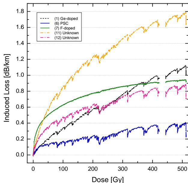
Figure 4: Induced losses in various fibre samples as a function of total dose in a high energy physics radiation field.
