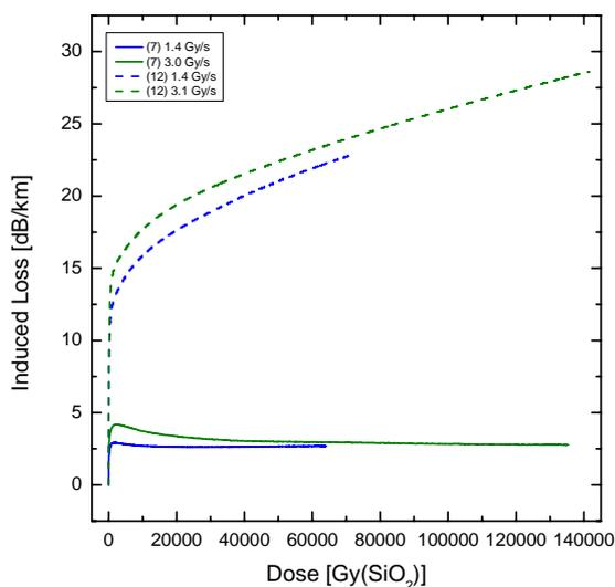
Figure 3: Induced loss for the two best performing fibres (sample#7 and sample#12) in the screening test at 1.4 Gy/s and 3.0 Gy/s.
