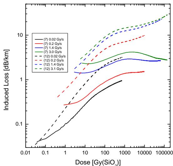
Figure 2: Dose rate dependence for the two best performing fibres (sample#7 and sample#12) in the screening test.
