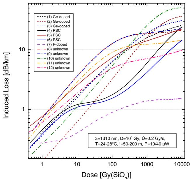
Figure 1: Induced loss as a function of dose for the fibre samples in the screening test.
