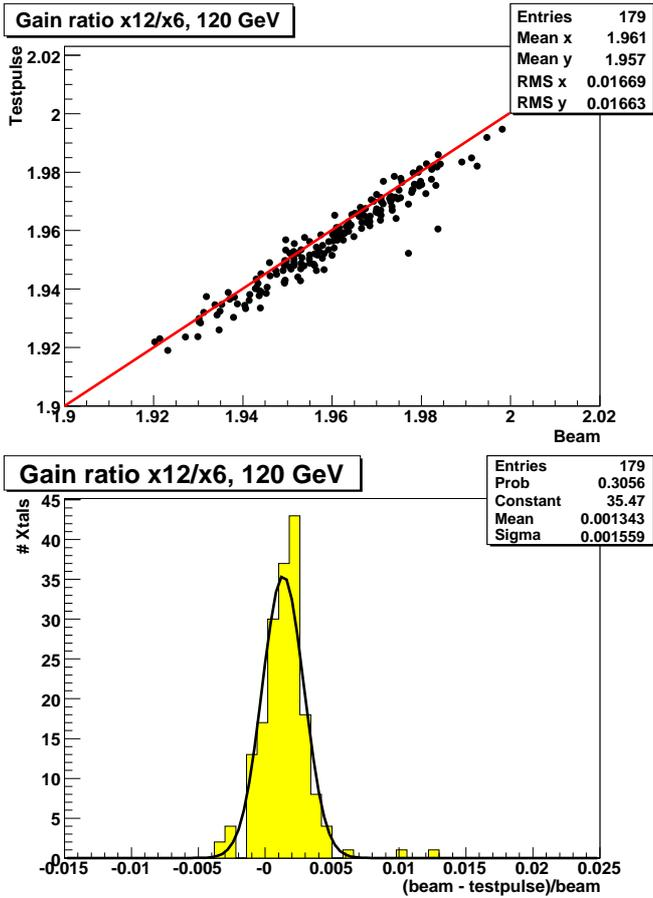
Figure 5: Correlation (left) and difference (right) between gain ratio 12/6 measured by the MGPA test pulse and with an electron beam of 120 GeV at CERN for 179 channels.
