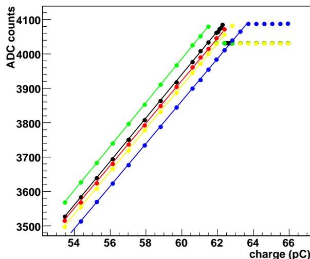
Figure 8: ADC output for different injected charge in a single channel (top) and linearity plot for five channels of the barrel VFE board (bottom).
