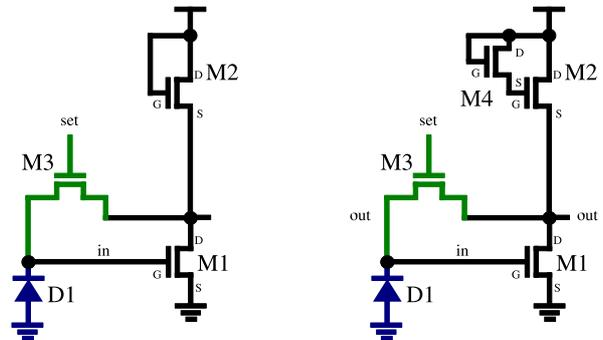
Figure 4: Amplifiers with time variant feedback. Left: standard schematic, right: improved schematic.
