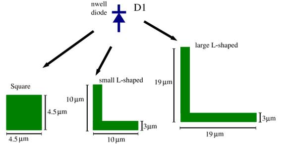
Figure 6: The layouts of tested diodes.
