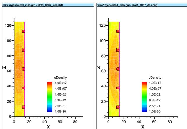
Figure 7: Electron concentration, in the p-substrate is due to energy deposited by m.i.p, shown after 19 ns: left not graded substrate, right graded substrate.
