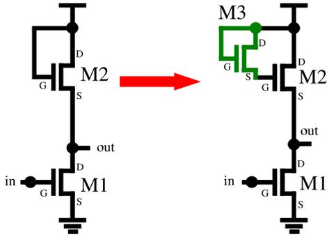
Figure 2: Standard (left) and improved (right) amplifier schematics.
