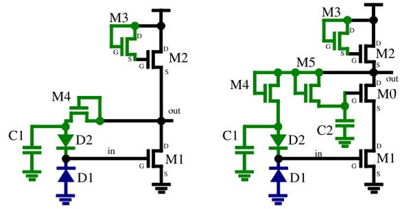
Figure 3: Common source and cascode schematics with feedback, the improved load use to increase the gain.
