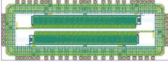
Figure 5: The layout of the test chip.
