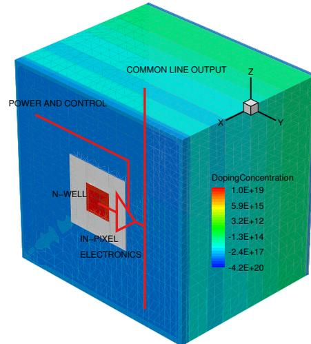
Figure 1: Basic pixel cell: nwell in p-type substrate, the readout electronics is placed in the substrate between the nwells.
