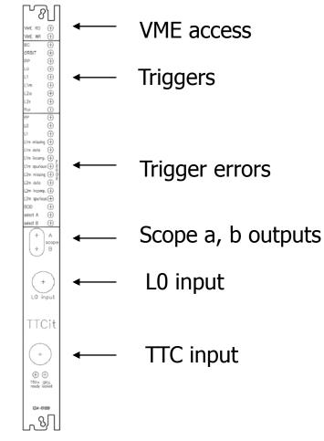
The TTCit can be added, temporarily or permanently, to the sub-detector TTC partition (LTU, TTCvi, TTCex, TTCit) or it could also be installed separatel
