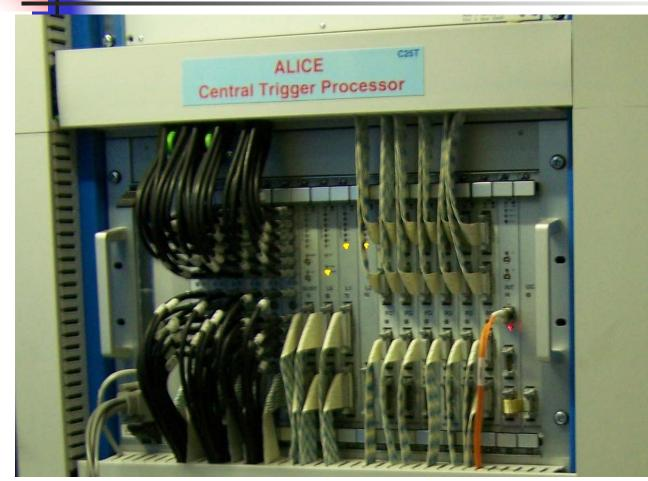
Due to short time for L0 latency the CTP is in the experimental cavern.
