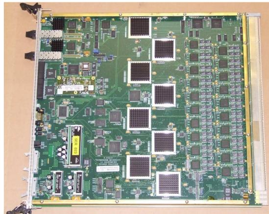
Figure 3: Example of a CPM processor module
