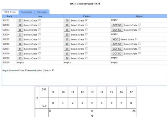
Figure 7: RCT Trigger Supervisor window for programming individual crate crates and cards. Individual tests can be chosen.
