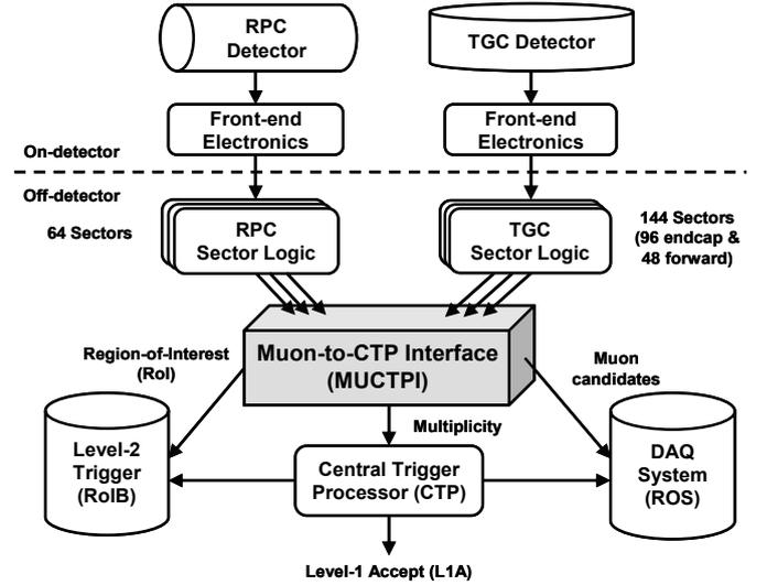
Figure 1: Overview of the ATLAS Level-1 muon trigger
