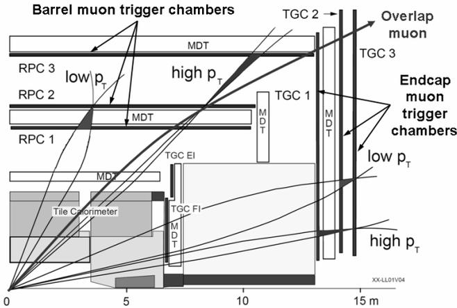
Figure 2: Barrel and end-cap muon trigger chambers
