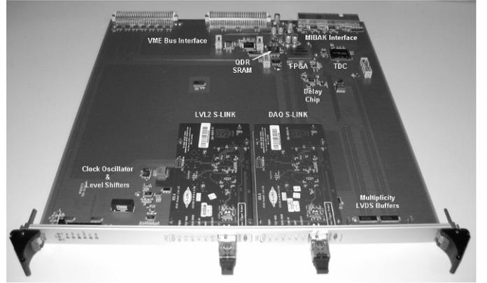
Figure 8: MIROD/CTP module picture
