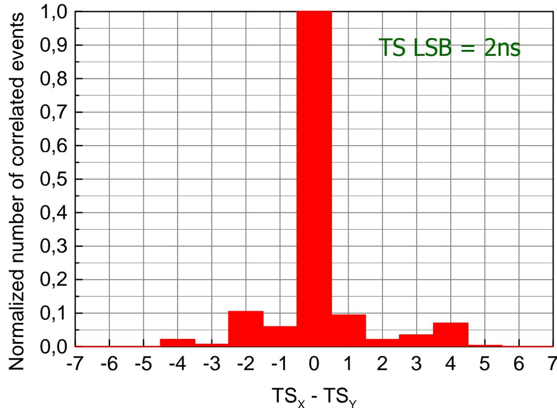
The histogram of Time Stamp coincidence between X and Y strips demonstrates the coincidence resolution of 2 ns as expected for the clock frequency of 128 MHz
