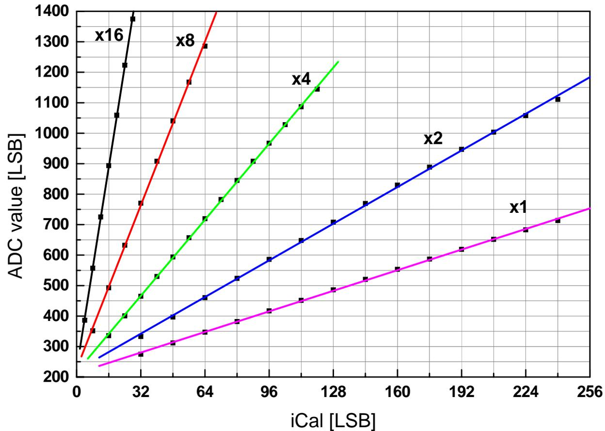
Measured gain factors:  $\times 1$ ,  $\times 1.78$ ,  $\times 3.70$ ,  $\times 7.94$ , and  $\times 19.58$
