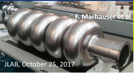
5-cell 800 MHz cavity, JLAB prototype for FCC-ee (top mode) & FCC-eh; also single-cell cavities for all FCC's
