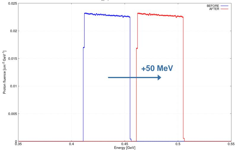
Proton energy spectrum before and after acceleration
