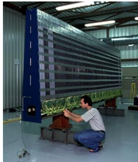
Tile calorimeter (CERN – ATLAS collaboration)
