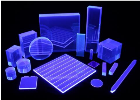
Scintillators (Eljen technology)
