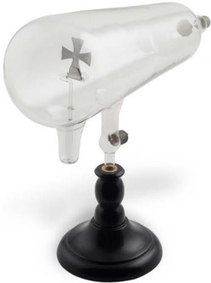
Tube de Crookes MHS 2235 Aluminium, bois, fer, verre, 19 e siècle
