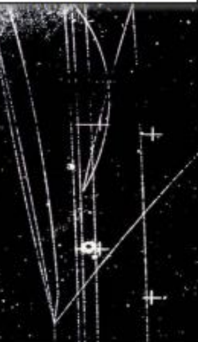
Particle colliding with a proton in liquid hydrogen A "Bubble Chamber"
