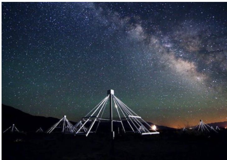
Large Aperture Experiment to Detect the Dark Ages (LEDA) at Owens Valley in California. (30-88) MHz.
