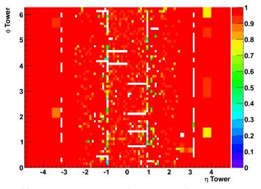
Problems at joins, e.g. Barrel to Ext Barrel at η = 1
