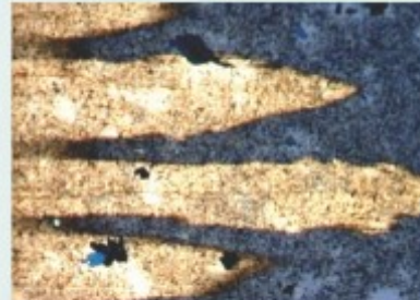
Picture 2. Formation of oxygenation cracks in YBCO MMS at annealing in oxygen at 400 °C
