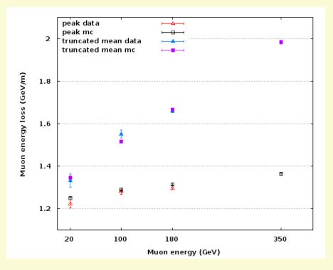
TileCal response to muons as a function of muon energy data compared to MC:
