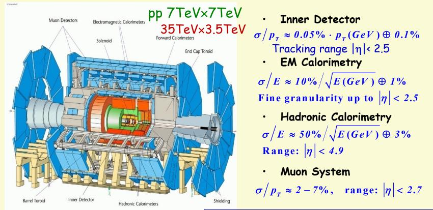
Magnetic field : 2T Solenoid + 3 air core toroids *start: autumn 2009* 27/05/2011 S. Tok Precision physics in  $|\eta| < 2.5$ Lepton energy scale: 0.02% (Z $\rightarrow$ II) Jet energy scale: 1.0% (W $\rightarrow$ jj)
