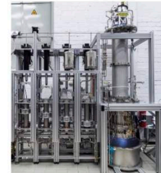
Rn distillation column for XENONnT (reduce 222 Rn - hence also 214 Bi - from pipes, cables, cryogenic system)
