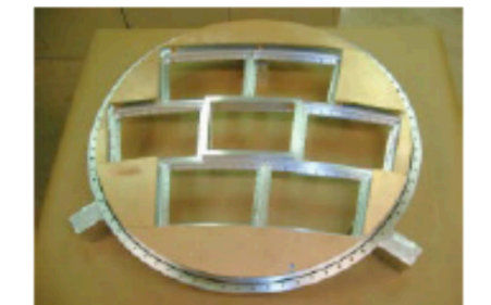
Triple-GEM r/o module for LCTPC
