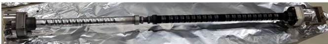
Cathode used for Ti + C deposition on the next FCC-hh beam screen prototype. Credit to P. C. Pinto and his team, in particular S. Fiotakis for making the coating.
