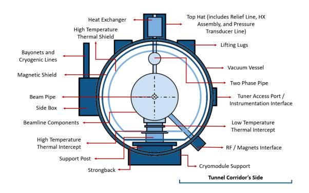
The "Strongback" serves as the coldmass foundation for PIP-II cryomodules.
