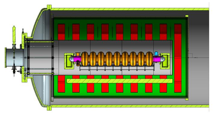
First and only Nb<sub>3</sub>Sn coating chamber capable of coating 1.3 GHz 9-cell cavities or 5-cell 650 MHz cavities
