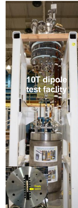
4.2 m, 1.8K Test facility testing AUP quadrupoles
