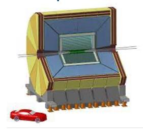
Full silicon vertex-detector+ tracker 3D high-granularity calorimeter Solenoid outside calorimeter
