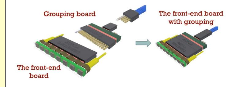
We should do a sum of current at the tail of the cable (from 16 pins to 2 pins). Ideas on how to proceed? What do we need?
