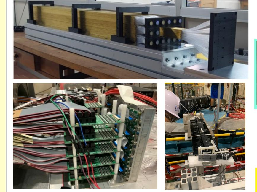
Examples of tests already performed by some collaborations to test the DR approach. The picture on the left shows the use of "bucatini" shape absorber and scintillating fibers as detectors.
