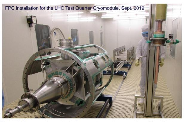
For LEP & LHC, FPCs were installed after cavity train was placed inside the vacuum vessel For FCC, it might also be interesting to have the option to install the FPC after cryostating. **Pros:**
