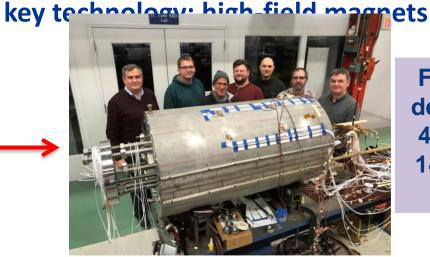
FNAL dipole demonstrator 4-layer cos 14.5 T Nb<sub>3</sub>Sn in 2019
