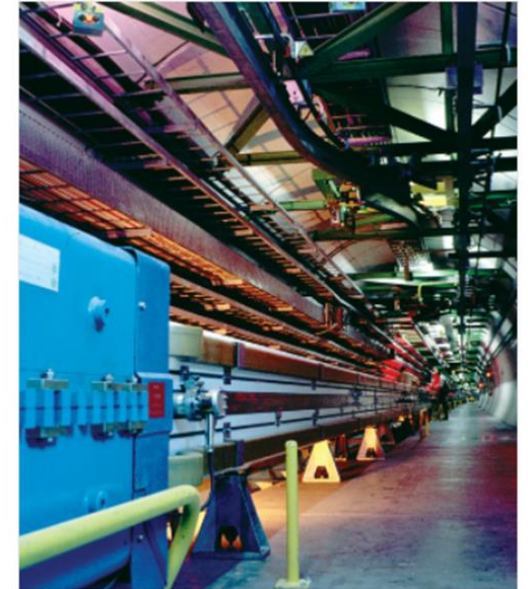
Focus and bend A quadrupole stands next to one of the long dipole magnets that curved electrons and positrons around LEP's 27 km-long ring. Credit: CERN
