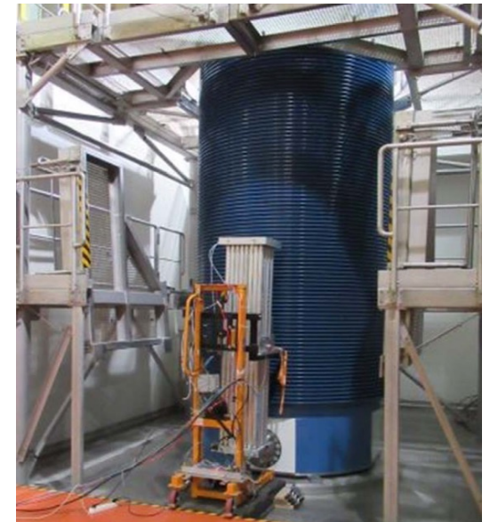
A small detector module prototype has been constructed and tested in the vicinity of a spent fuel cask
