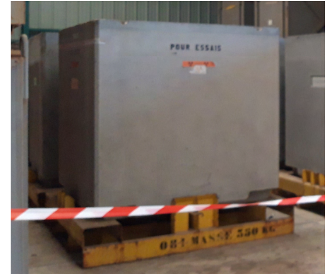
IP2 Type containers 1.7 m side (5 m 3 ) 12 tonnes overall weight
